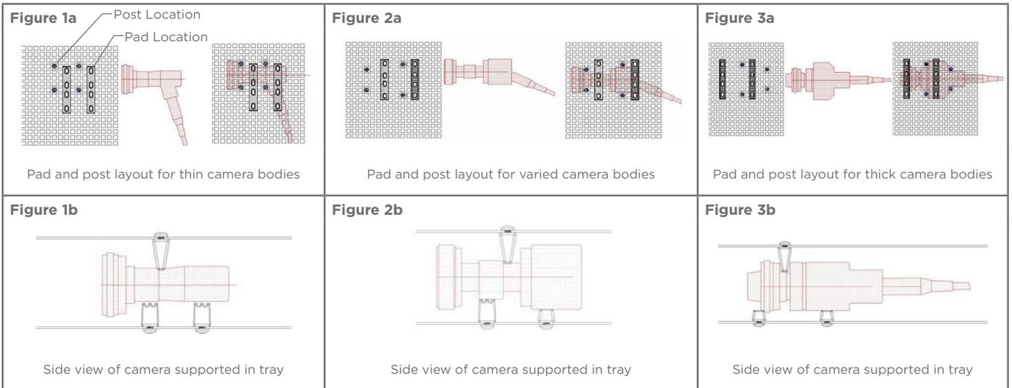
5. Place IN-6870 on top of the camera using figures 1b, 2b, and 3b for orientation and suggested locations. IN-6870 holds the camera in place when the lid is on the tray.
